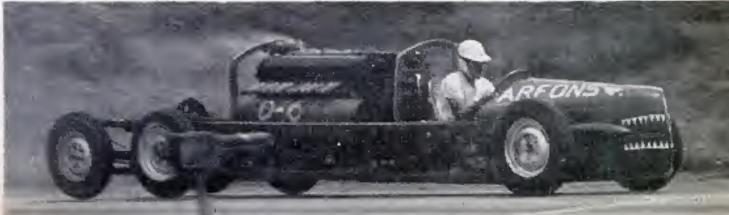
Tandem-wheel drive increases the traction and minimizes the tendency to "fishtail." Car has a clutch from a 30-ton tank
